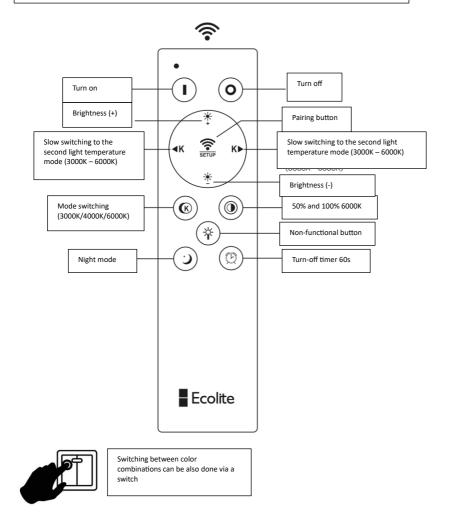
The lights are already paired with the remote control by the manufacturer. If the remote control doesn't communicate with the light, pair them.
